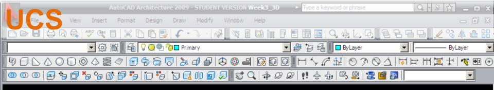
The UCS system (User Coordinate System) allows us to redefine where our drawing plane is.
